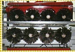
Transverse working cleaning aggregates, consisting of an oscillating four brush unit. On demand top and bottom units.
