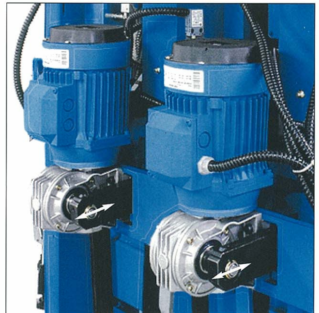
View of the oscillation system of brushes S-250
